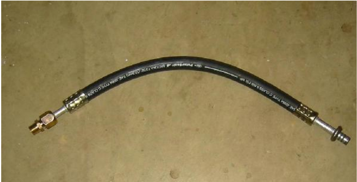
Update Aug 08: New discharge hose, new fitting for the compressor. The suction hose is very difficult to seal on a smooth piece of pipe, as shown above. I had this new hose and fittings made up locally.
