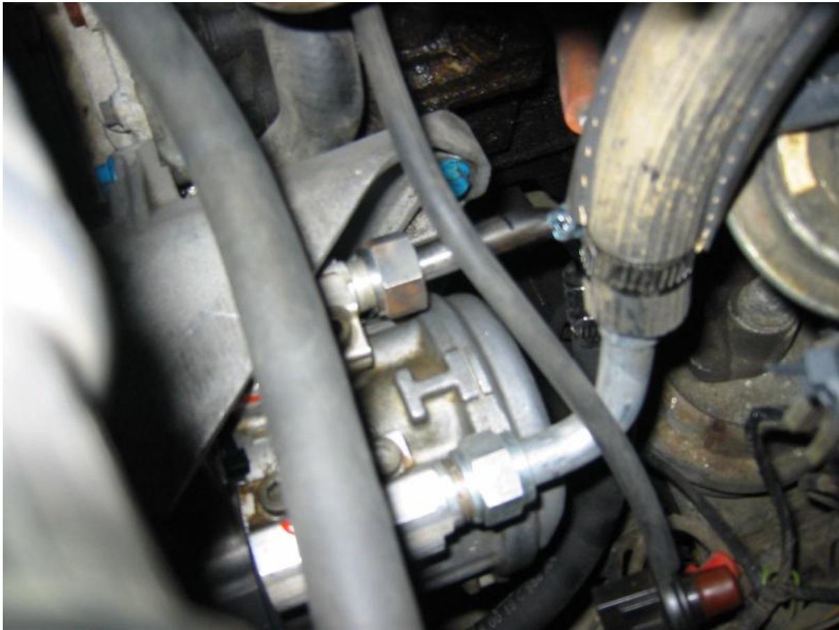
Update Aug 08: New discharge hose, new fitting for the compressor. The suction hose is very difficult to seal on a smooth piece of pipe, as shown above. I had this new hose and fittings made up locally.
