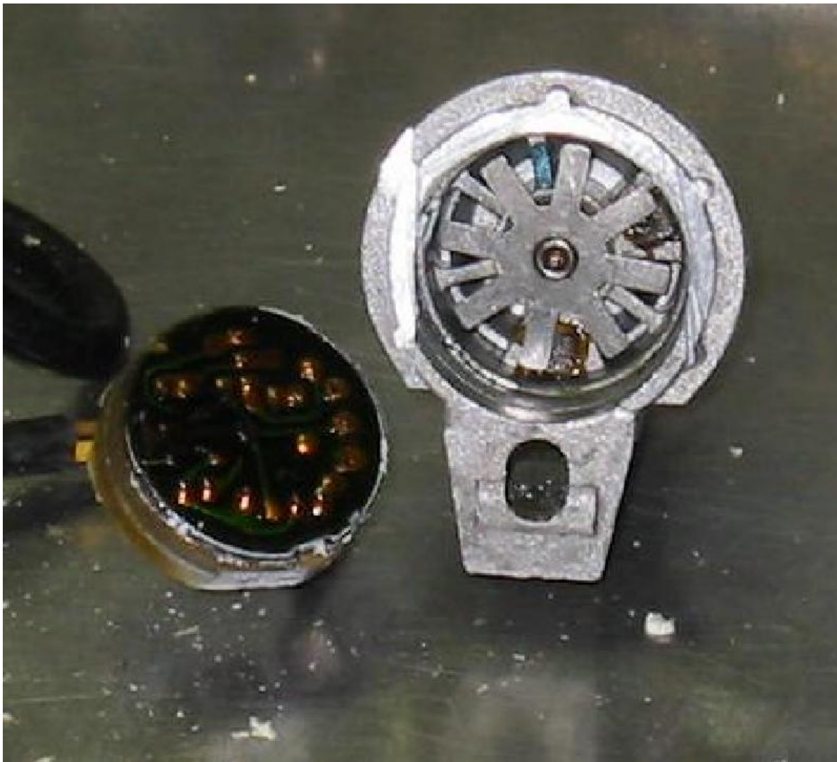
The transistor is shown at about 9 o'clock on the circuit board. The magnet is visible at about 6 o'clock behind the vanes in the body.
