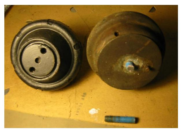
The motor bracket needs about a half inch shaved off the top to match the length of the stud on the new mount. It also needs to be drilled out a little for the stud and the locator pin.
