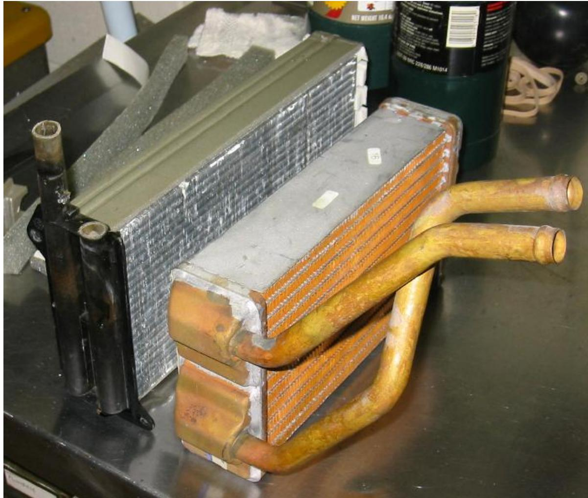
It also obviously needs work on the fittings. Here's my fix. I cut pieces from the new core. They're stout and take some time to solder. Wire-wheel clean the cut ends to make the solder stick. Use plenty of flux.
