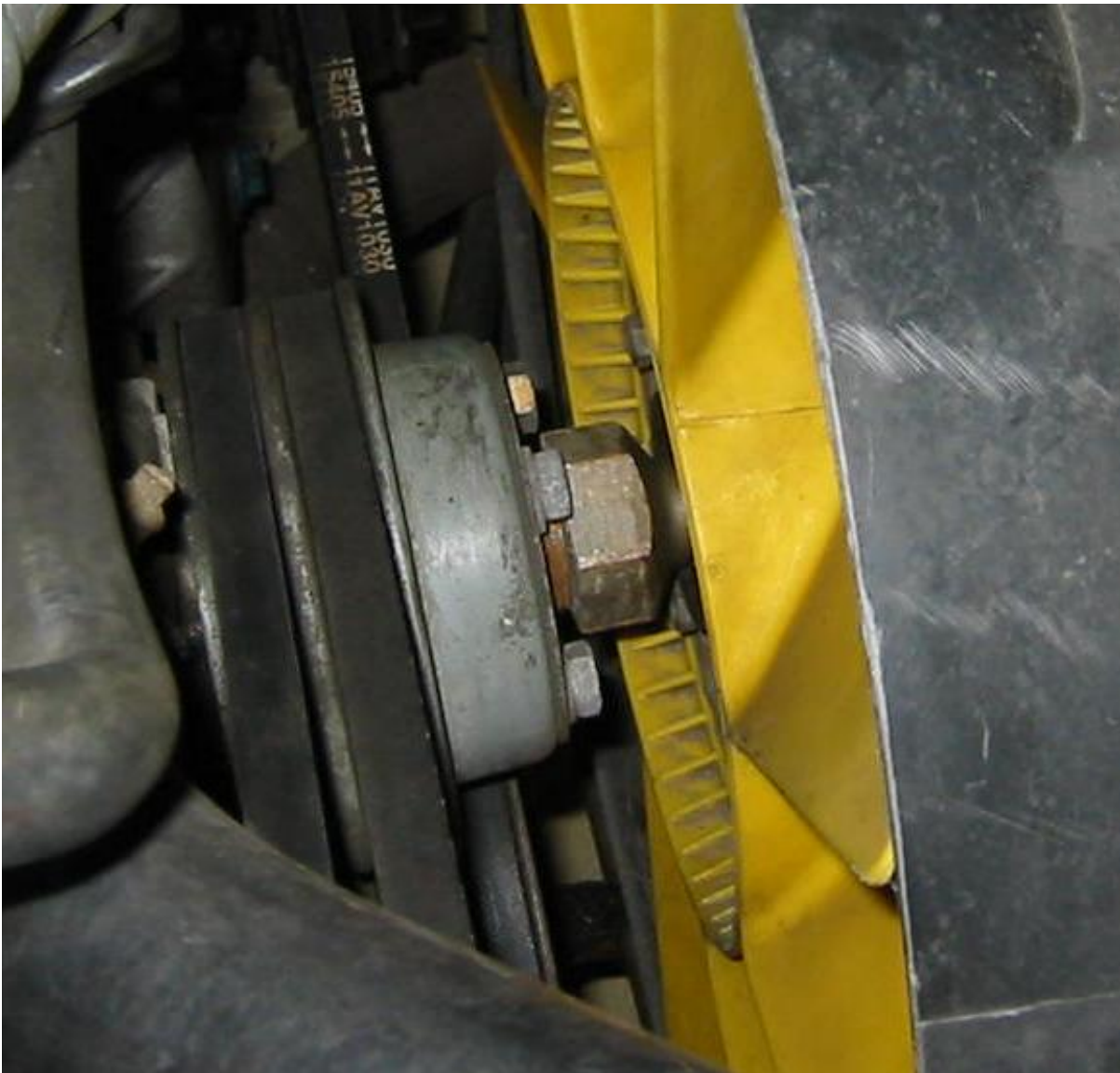
This is the Bronco II/Ranger clutch on the car. Notice the extra space available to remove it. Even with the extension, it clears the radiator on removal with no problems.
