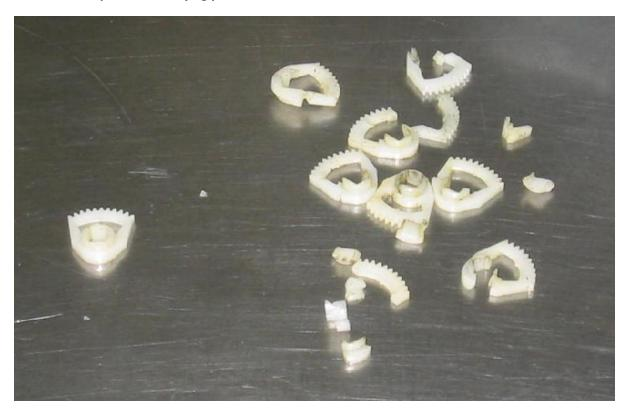
Here's the center door flap after being abused by the motor:
