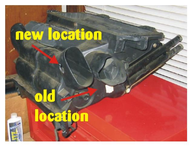
The upper air valve/air temperature door sometimes leaks air, blending warm air with cool air. Not good on hot days.
