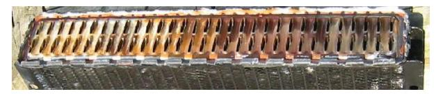
There's a flat seal/o-ring between the tank and the core (not pictured).
