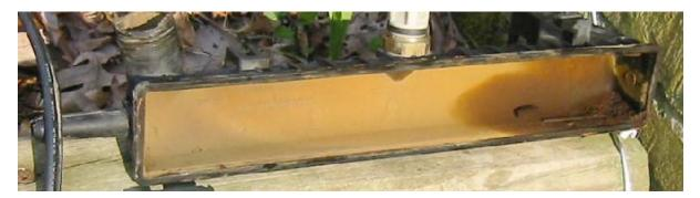
Clean the gasket. While you're in there, run a smoothed-off band saw blade through the tubes. Amazing how much difference it makes in keeping things cool. If yours is original, it might be too fragile to rod out.
