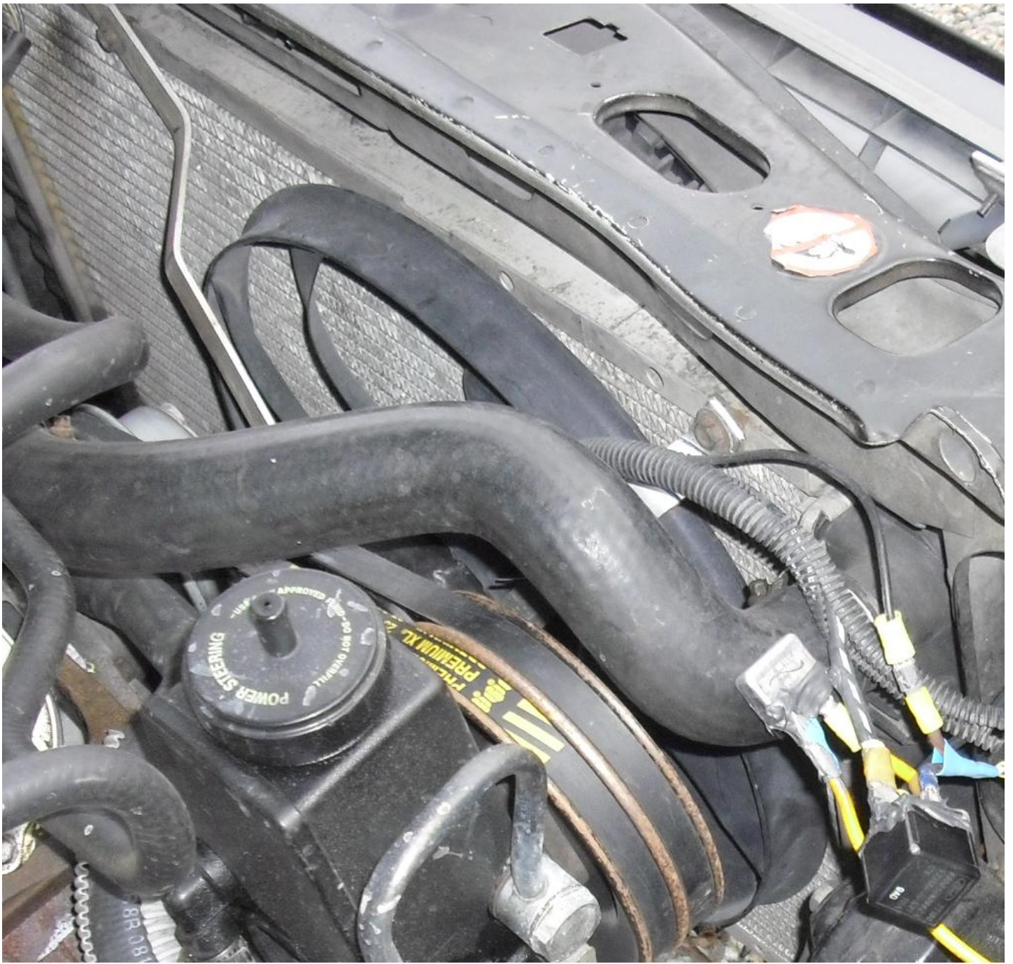
As shallow as the fan motor is, it still needs to be offset from the water pump.
