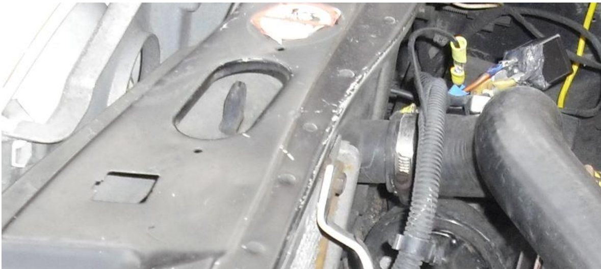
As shallow as the fan motor is, it still needs to be offset from the water pump.
