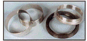
Rebuilders should always cover the factory seal with a sleeve Ford offers a kit with a seal and a sleeve (right), but most rebuilders prefer to use a sleeve from Micro Sleeve or Classic.
