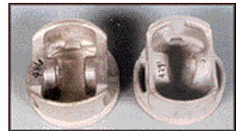
The latest piston (right) that came out in '98 is 50 grams lighter than the one used in the '97 engines. The pin bosses are closer together, the skirts are thinner and there are cavities behind the ring lands to reduce weight.
