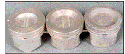
There have been three pistons used in the 4.0L. The original design (left) had a shallow dish, the second version (middle) had a deeper dish to compensate for them smaller, heart-shaped chamber, and the latest design (right) had a similar dish, but it was milled squared-off in the bottom.
