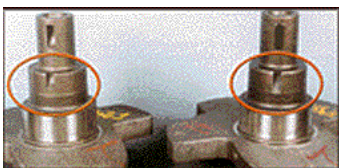
The length of the notch machined in the step was changed in '95. The notch in the 95TM-AB (left) was shorter than the one in the 95TM-AA. Both of these cranks are interchangeable.
